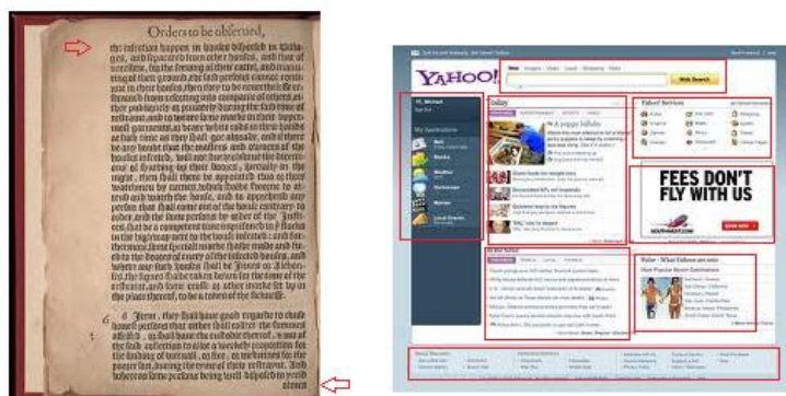
Figure 32: Typical examples of a book and web-site page. The book-page has one entry/exit point, marked by the red arrows. In the web-page the red squares mark clusters of different entry/exit points.
